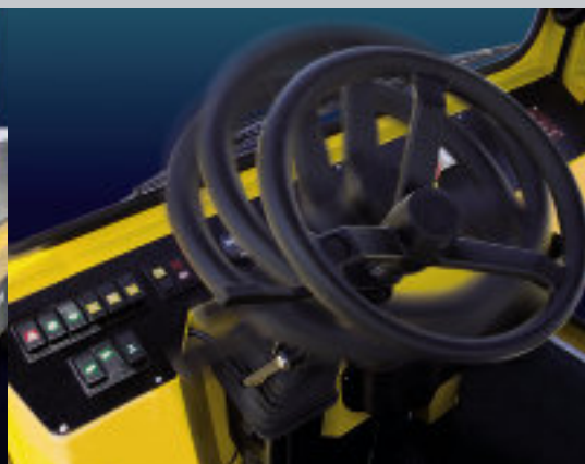
Multi-adjustable steering column
