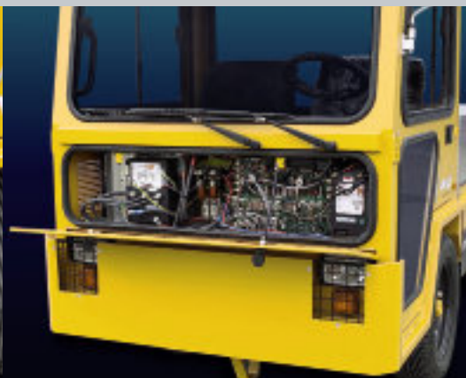
Drive components arranged in a service-friendly manner
