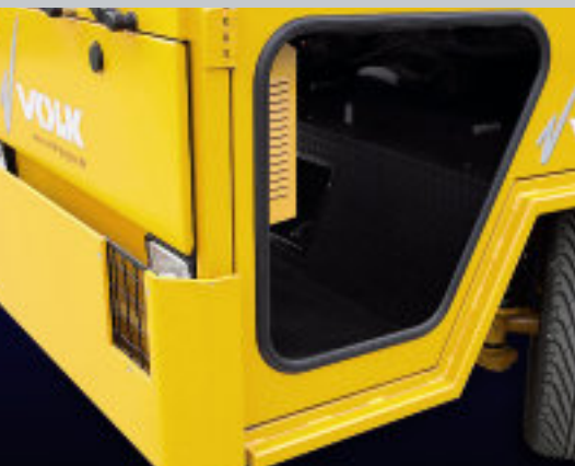
Window in the foot area
